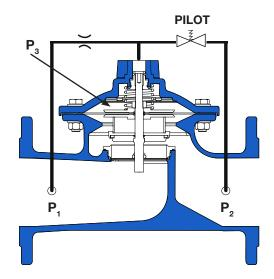
P<sub>1</sub>: Inlet pressure/upstream pressure
