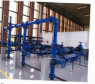
The flow lab is primarily intended for the development of new products and for testing existing products. The lab is used for testing valves and actuators under various conditions. The lab is a key part of AVK's commitment to quality and innovation. The lab is a key part of AVK's commitment to quality and innovation.
