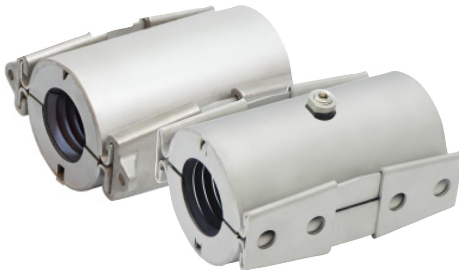
The new Quick Repair (QR) transition coupling sets a new standard for quick but professional repairing of leaking pipe connections. AVK Nederland has two types of couplings, one for water and one for gas. The QR transition coupling is maintenance free and made entirely of stainless steel with a rubber sealing inside and is therefore fully protected against corrosion.
